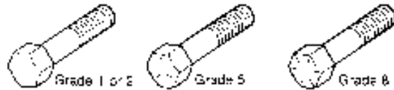
Figure 5: Grade Markings on Bolts
